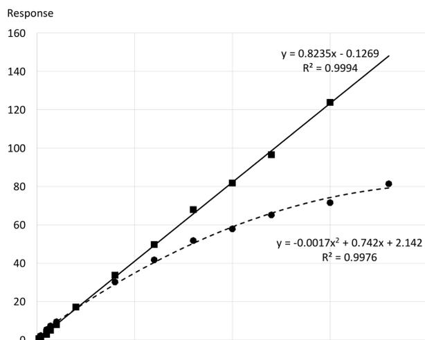
**Figure 3.** Calibration of triclosan with standard parameters for the internal standard (triclosan-D<sub>3</sub>, 50 mDa mass window, m/z 289.9622), ●, and with a narrow mass window (10 mDa) and <sup>37</sup>Cl isotope peak (m/z 291.9592) ■. Response =  $\text{Area}_{\text{TCS}} \cdot \text{Concentration}_{\text{TCS-D}_3} / \text{Area}_{\text{TCS-D}_3}$ .
