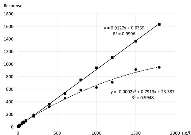
**Figure 1.** Calibration curve of carbamazepine with carbamazepine- $\text{D}_{10}$  as the internal standard ● and linear calibration with carbamazepine- $^{13}\text{C}_6$  as the internal standard ■. Response =  $\text{Area}_{\text{CBZ}} \cdot \text{Concentration}_{\text{ISTD}} / \text{Area}_{\text{ISTD}}$ .
